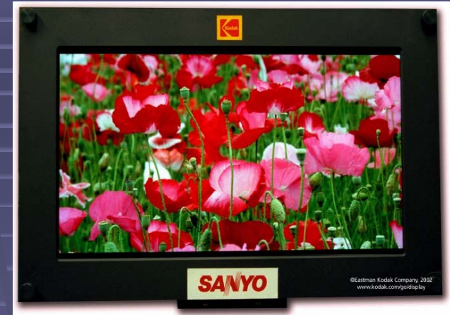
15" full color AM display by Eastman Kodak Co. and SANYO Electric Co.
